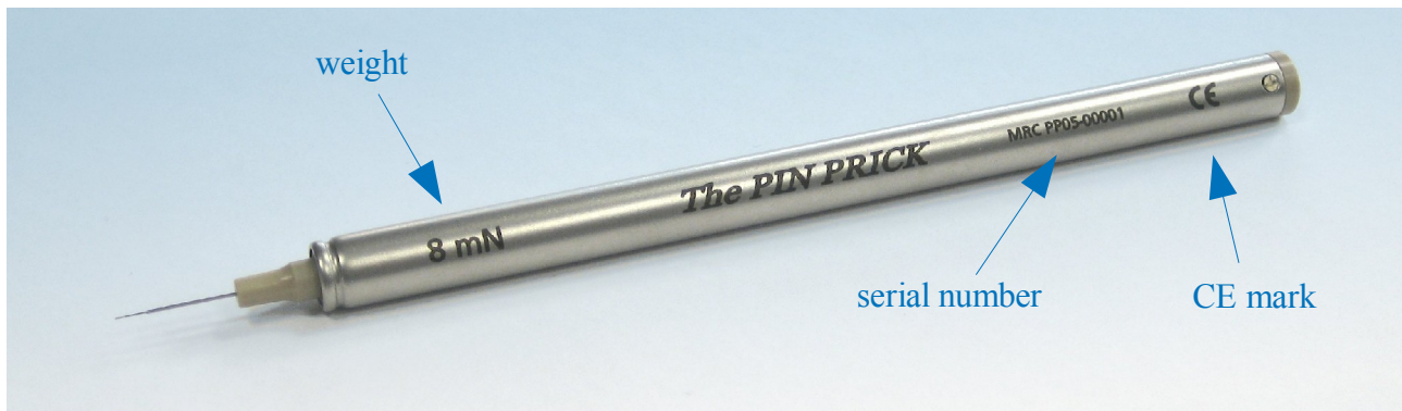
Figure 5: Marking of a PinPrick stimulator
