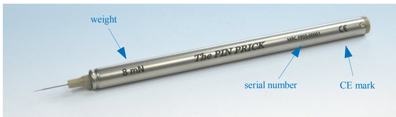
Figure 5: Marking of a PinPrick stimulator
