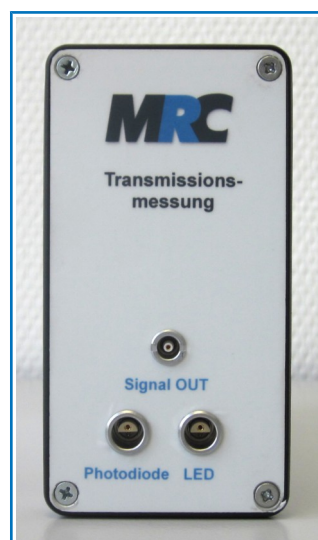
Figure 5: Electronic box of the transmission meter with fixed adjustments
