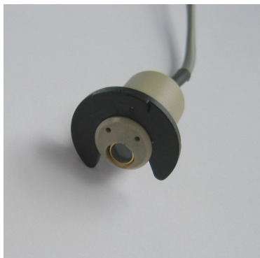
Figure 2: UV photodiode in plastic fitting with fixation clip. Further, a temperature sensor is mounted to the clip (not mounted in the photo).
