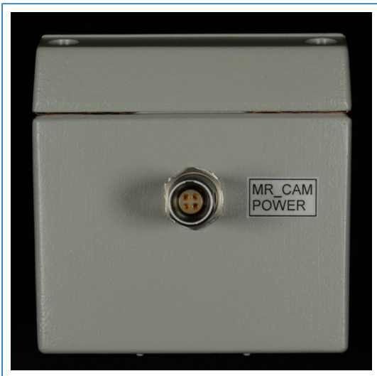
Figure 4: Filter box (front side)
