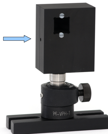
Figure 14: 4-quadrant-diode. The arrow points to the potentiometer for intensity variation (Please use a screwdriver)
