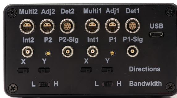
Figure 25: Right panel with additional “Adjust-in” inputs for x and y position of two PSDs
