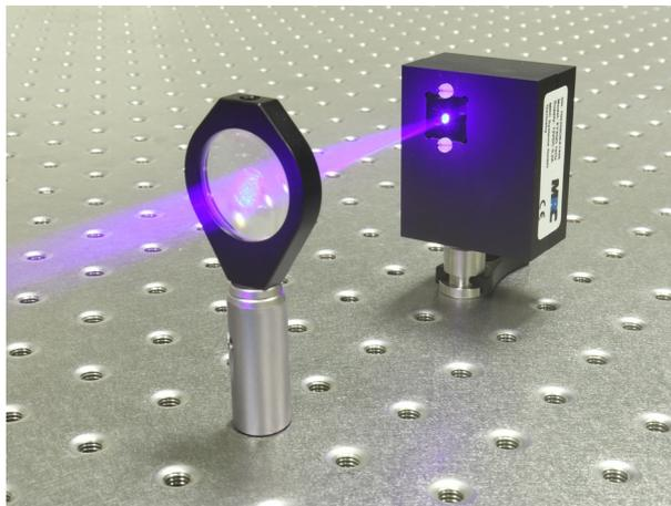
Figure 1: Use of a lens to reduce the beam on the detector
