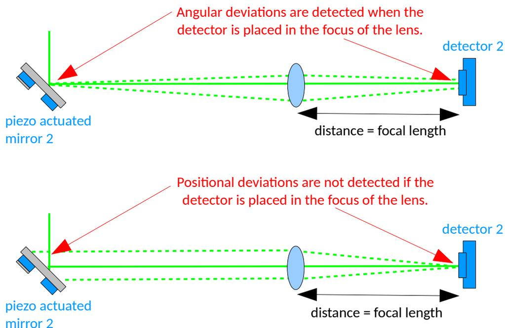
Figure 5: Effect of a lens on angular deviations (upper figure) and positional deviations (lower figure)
