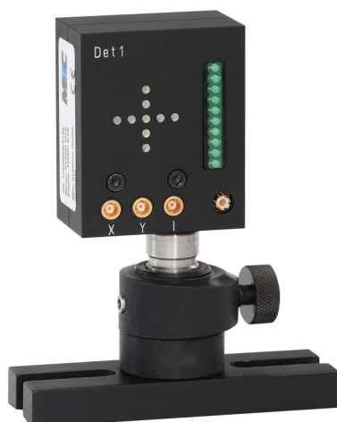
Figure 1: Rear side of 4QD detector (The base plate is not included in the delivery.)
